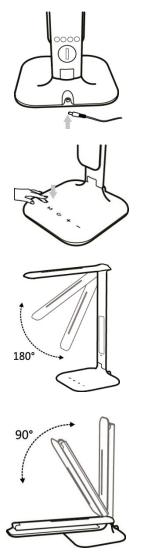
Connect the input connector of the power source to the input port of the table lamp. Then connect the charging adapter to the electrical socket.
